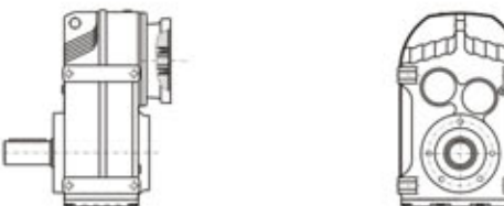
TF (TFF, TFA, TFAF, TFAZ) ...Y... 电机用户自配或配特殊电机时需加联接法兰 When equipping the user's motor or the special one, the flange is required to be connected
